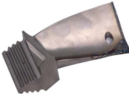
Blade in Process of Repair
