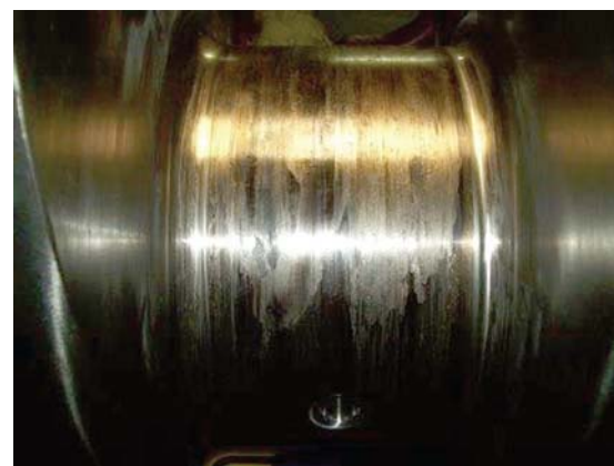
Damaged crank pin journal
