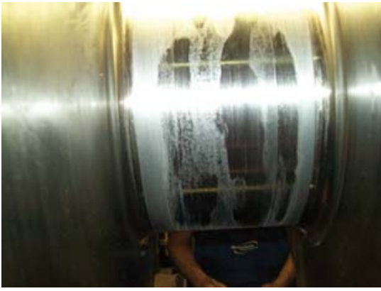
High hardness areas after machining
