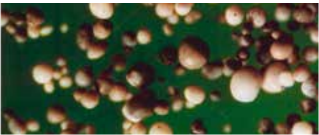
Catalyst residues (catalytic fines)
